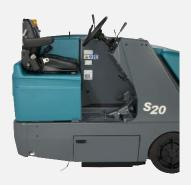
Spacious operator compartment incorporates adjustable seat, propel pedal, and steering column to customize fit. Important design safety features include excellent sightlines, side brush visibility, all levers forward sweeping, parking brake on light alert and much more.
