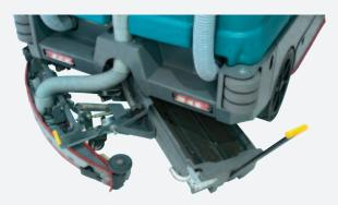
EasyRemove debris tray glides in and out on wheels, relieving operators of strain during transport and dumping, and increasing uptime.
