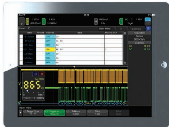
Figure 37: Tablet virtual front panel control.
