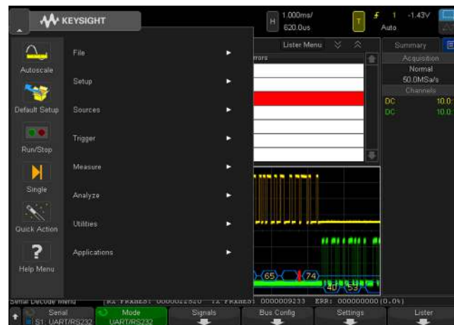
Figure 14: Use the Keysight pull-down menu for Windows-like operation.
