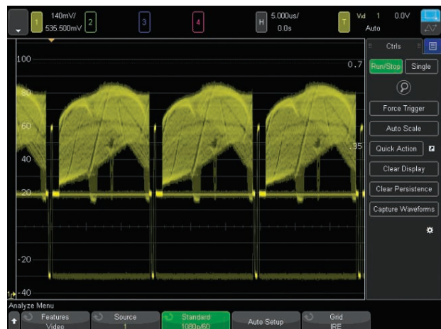
Figure 26: Triggering on 1080p HDTV signal analysis.
