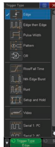
Figure 42: Wide array of advanced parametric trigger modes.
