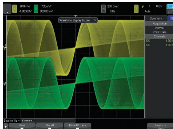
Figure 43: The "freeze screen" feature keeps the intensity-grading information while stopping the waveform acquisition.
